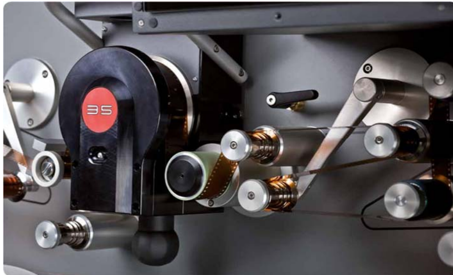
Figure 23 A part of the film path in DFT's Scanity. On the left side the film passes over the rounded gate. Source: DFT Scanity data sheet
