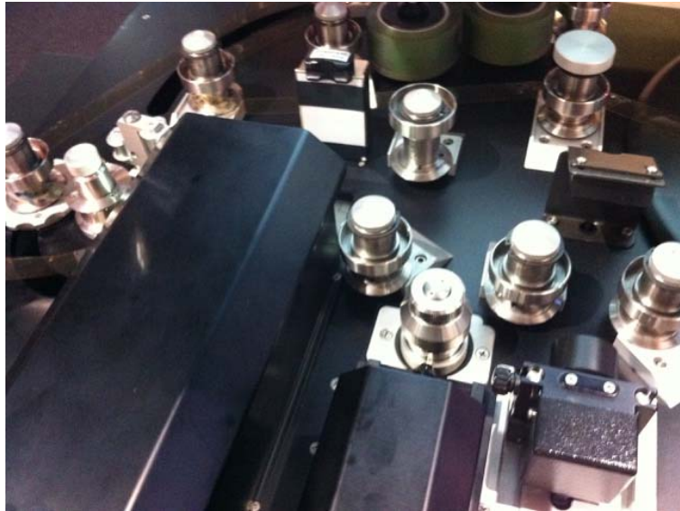
Figure 53 The diffuse flashing LED light source of the D-Archiver Cine10-A and the camera unit (covered)
