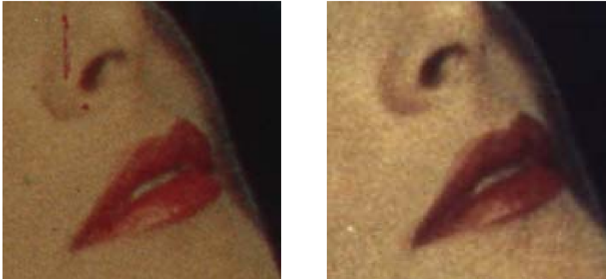
Figure 57 Comparison of scans on the Scanity, 2K at Sound and Vision in Hilversum (left) to the D-Archiver Cine10-A captured by Reto Kromer, also 2K (right) shows banding artifacts in the texture of the Technicolor film
